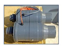
As the powder enters the larger volume of the filtration unit velocity drops and the powder falls to the bottom of the unit. The air is then drawn past the 2 filters, to remove any airborne powder.
